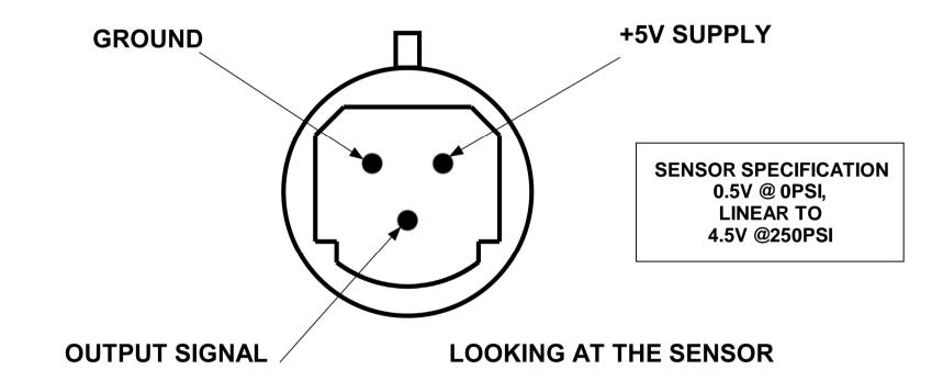
NOTE: INSERT WIRE THROUGH CONNECTOR FIRST, CRIMP THEN PULL BACK TO LOCK IN PLACE
